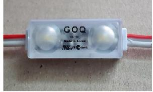
Most Preferred Best seller LED module : CE, UL, RoHS Certified Power Consumption : 0.72W LED provided by SAMSUNG SMD LED mounted : Made in Korea LED Driver : Constant Voltage Driving System Max. 50 modules in series Design of a new and unique CAP TYPE Optical Lens Each unit can be used to cut. Best Viewing Angle : **160°**
